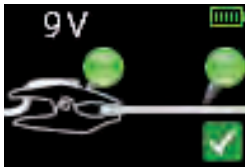
Grounding clamp detected, Coating without defect
